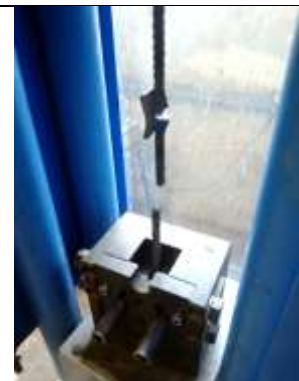
Rebar may break before the welded connection
