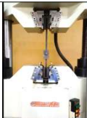
Testing 12mm rebar/30x6mm flat bar welded connection
